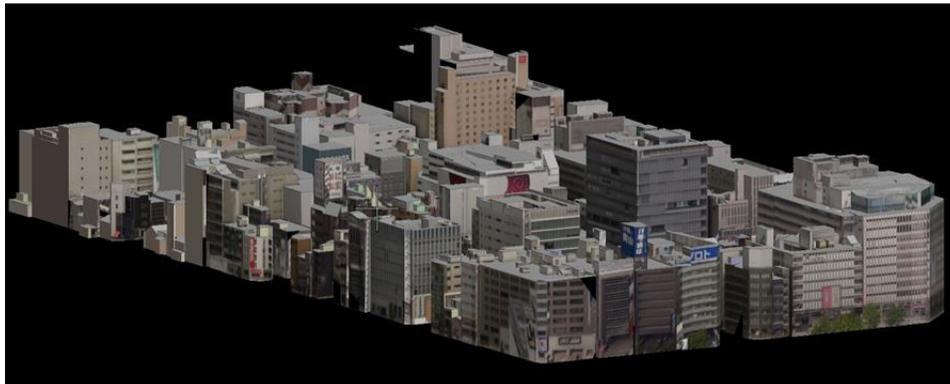
Figure 4: Oblique imagery rectified on building wall vectors
