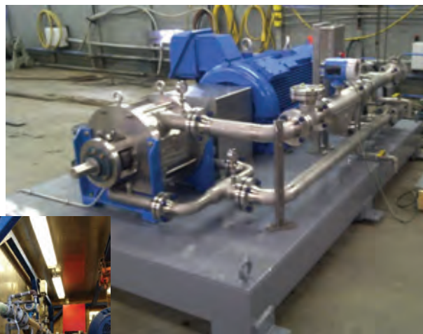
TrueMud Shear Mixer "Drop-In" Unit on a 8 by 10 Foot Skid.
