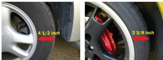
the greater the slip angle. As tire manufacturers built in more grip to the tires, they ran into an issue of having the tires roll off the wheel rims. The answer was to reduce the side wall height (or aspect). The photos show the aspect, measured in inches, for a GMC Envoy (4½”) and a Porsche Boxster (2 3/8”).
