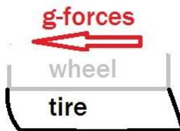
Tires are air filled rubber balloons around the wheels. The rubber flexes up and down, which absorbs road imperfections and the like. It also flexes side to side. The more friction induced in a turn, the more the flex. The diagram to the left gives you an idea of a cutaway view at the “Contact Patch”, where that portion of the tire is in contact with the road.
