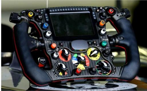
Here is a picture of a Formula 1 racing steering wheel. And you thought your radio controls on the wheel were a bother! The F1 drivers must use the 9 & 3 “racing” grip, which is in yellow on the Porsche wheel. It is the grip I use on track. It affords the most control in case of a blow out or an off track excursion. Since the hands are forced into opposite directions (one up and one down), it is much easier and quicker to bring both of them back to straight. The problem
