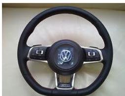
The first would be if the wheel has a flat bottom, like the VW wheel on the left. You could end up grabbing nothing but air as the wheel is turned. Also, as you let the wheel slide through your hand as you straighten out, it may be unsettling as the flat bottom passes.
