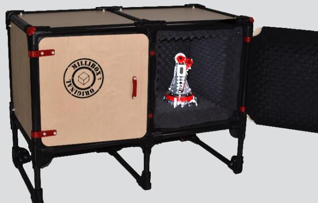
**MODULAR-** MilliBox chambers are built of modular construction components allowing the creation of several configurations to address differing needs. The MBX0x series is made of 60cm (24") cubic modules and the MBX3x series of 80cm (30") cubic modules. The chamber size is selected to satisfy your far-field requirements, and extension "cubes" can be added later if the need arises.
