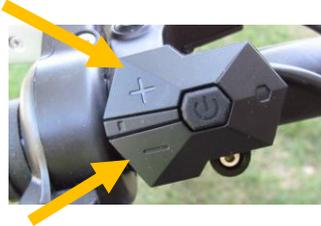
**NOTE: Do not engage throttle when not on bicycle as it will cause bicycle to thrust forward.**
