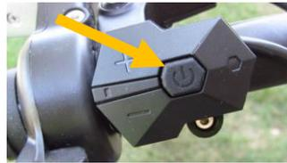
**Turn System Off.** Holding the Power Button another two seconds will turn the system OFF.
