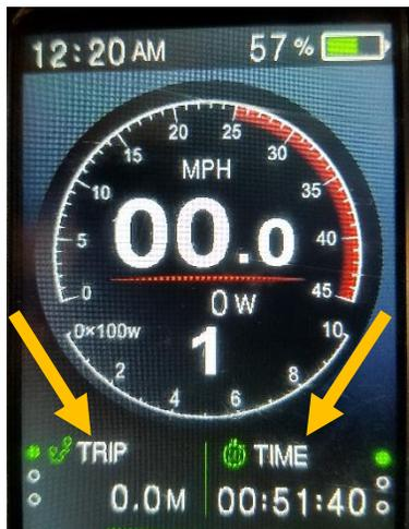
**Screen Settings.** When you turn the system ON, **Trip** and **Time** will be the default settings at the bottom of screen. Press the Power Button once, **Trip** will change to **ODO** (odometer). Press again and **ODO** will change to **Range** (miles you have left). Press Power Button again and screen will return to **Trip** and **Time**.
