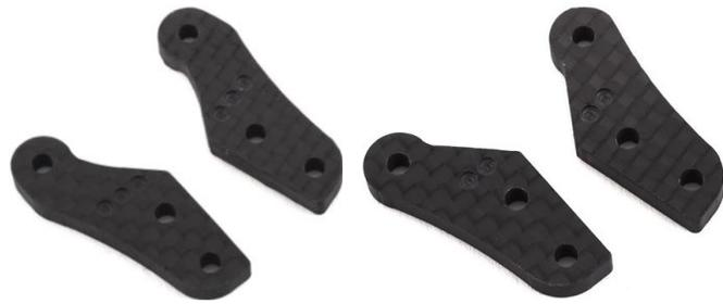
Steering plates are identified by number of indents on the plate
