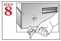
After filling dishwasher for the first time, **(CAUTION: turn power supply off)** reconnect the factory unplugged wire to booster high-limit switch located behind front panel.
