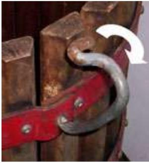
3. Once retaining pin is properly inserted into steel bands, rotate downwards, or clockwise.
