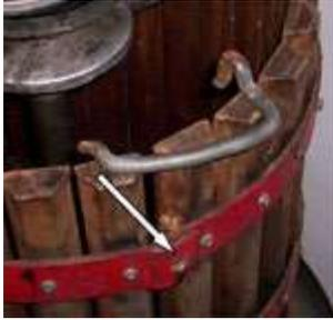
1. Insert slightly bent end into steel band.
