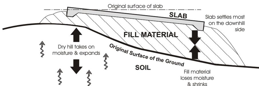
**Fig. 2 TILTING OF A SLAB ON A HILL**
