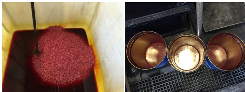
Photographs show (left) chromium trioxide flakes with addition of water to reduce dust during mixing and (right) empty drums
