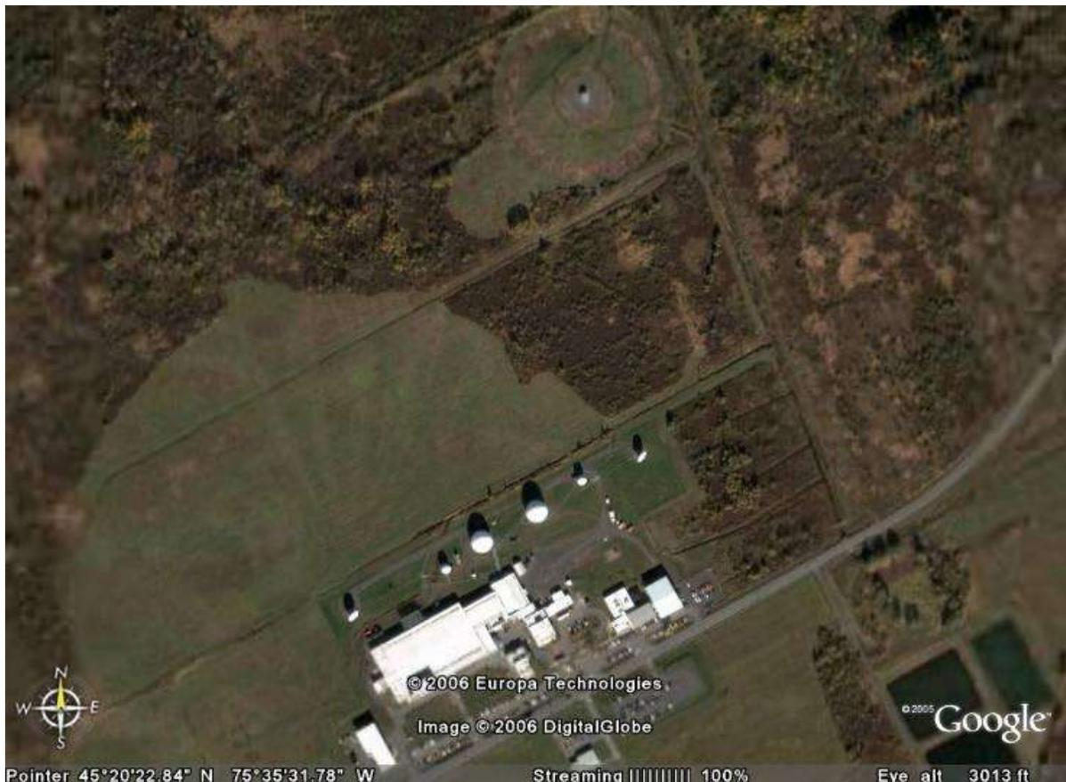
The above 'satellite' view (before construction of the 'bypass'), from an altitude of 3,000 feet, shows the main buildings, the radomes and in the upper center, the Pusher antenna. The Pusher system is designed for the interception, monitoring, direction-finding and analysis of radio signals in the HF band from 1.5 to 30 MHz *communicated in plain language.*
