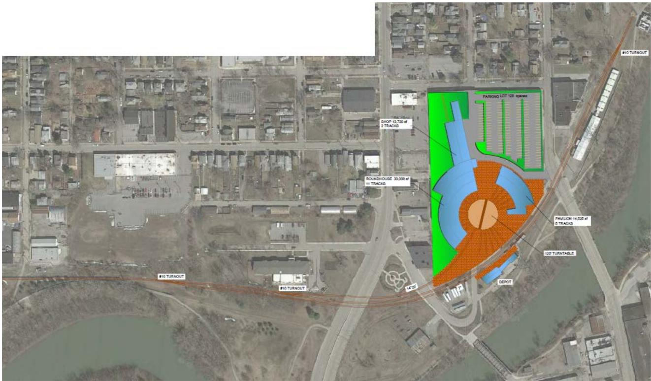
Note that our rendering extends well beyond the proposed site, to include the turnouts and additional trackage necessary to access the site with a full train. Curvature was generally feasible, except for the placement of a curved switch onto the site in what was essentially the middle of a grade crossing. Our design moves this turnout further west; it was also discussed if this turnout could be relocated to the northeast side to reduce moves across high-traffic streets to a lower-traffic street.
