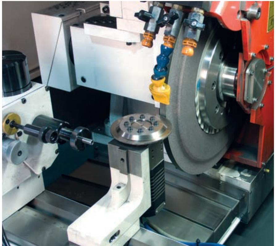
Hi-Quality Carbide employs the S33 grinder's rotary disk dresser to maintain a radius on the corners of flat grinding wheels, and uses those corners to profile complex contours on carbide punches
