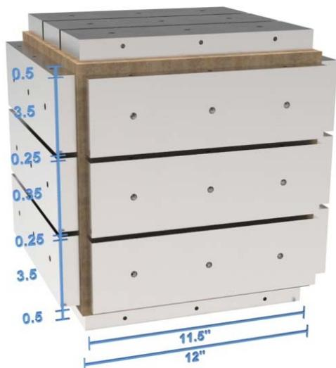
Figure 2. Loading plates on cubical specimens
