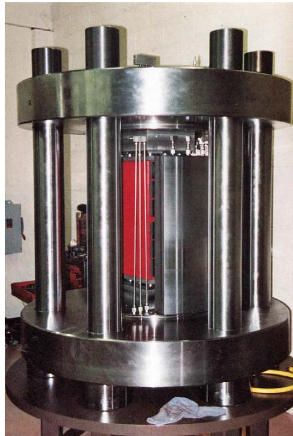
Figure 6. RPS Poly-axial system for 300mm x 300mm x 600 mm specimens
