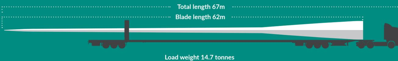
Each wind turbine blade is 62m long and weighs almost 14.7 tonnes. The size of the blades allows more wind to be captured – meaning higher amounts of clean energy can be generated.
