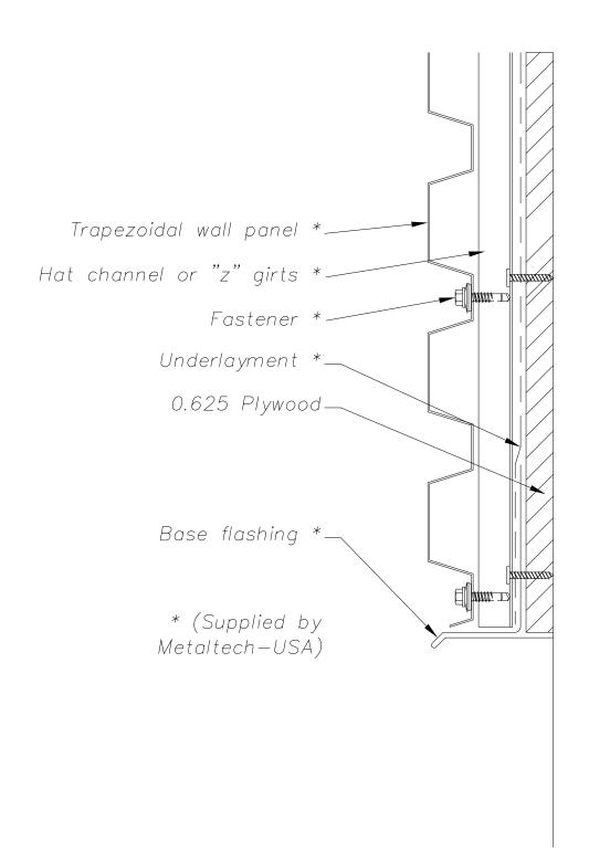
NOTE: Base flashing not to exceed 1.75 inches unless installed with a stiffner
