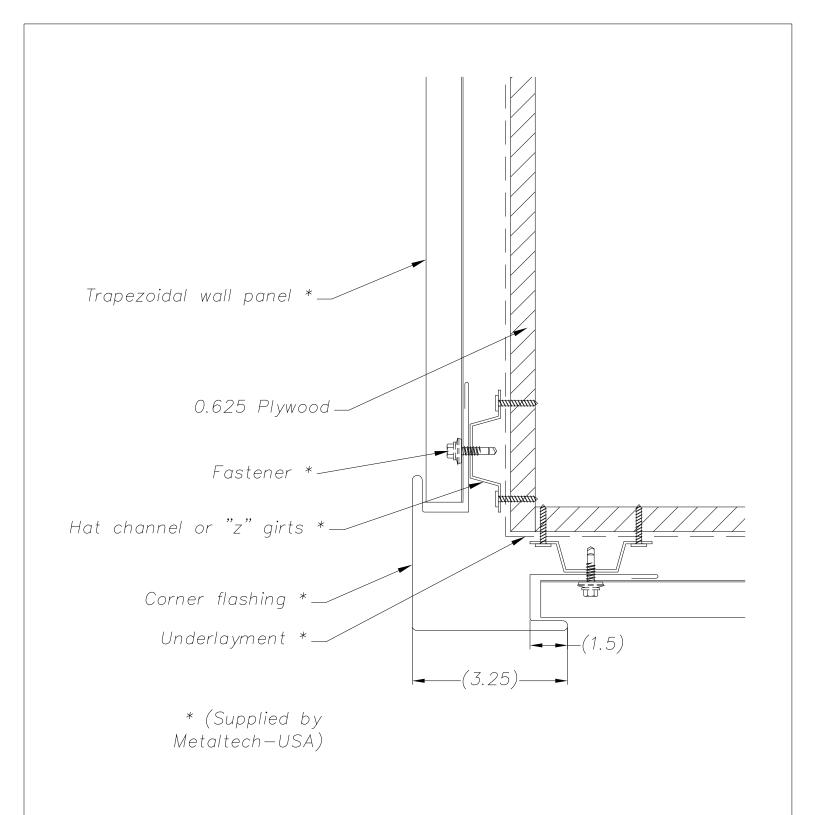
NOTE: Minimum difference between exposed corner width and pocket depth equal 1 3/4"
