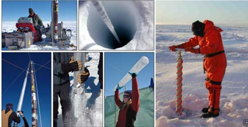
(Clockwise from top left) Ice coring machine, hole in ice, pulling ice core from machine, man with hands on ice core tube in ground, scientist holding up ice core in triumph, man hand drilling ice core.
