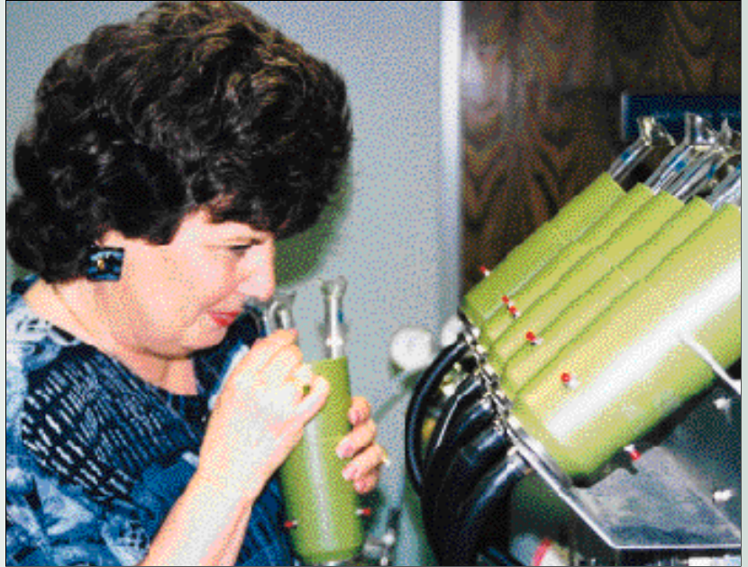
Using an olfactometer, Brown and Caldwell employee and volunteer odor panelist Sharon Parmalee tries to distinguish a diluted foul-air sample from samples of odor-free air.
