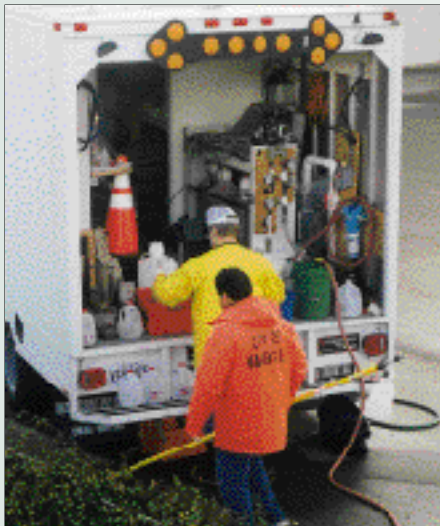
During an assignment to test flow measurement at the City of Vacaville, Calif., wastewater treatment plant, Thayne Loendorf, engineering technician from Brown and Caldwell's Portland, Ore., office, assisted by a member of the plant's operations staff, prepares background samples using one of Brown and Caldwell's specially outfitted vans.
