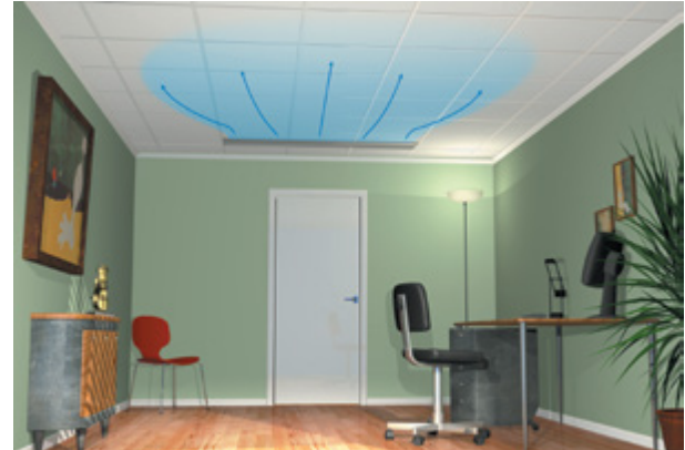
Picture 5. Polaris S-30 installed at the ceiling's rear edge, with air injection across the ceiling.
