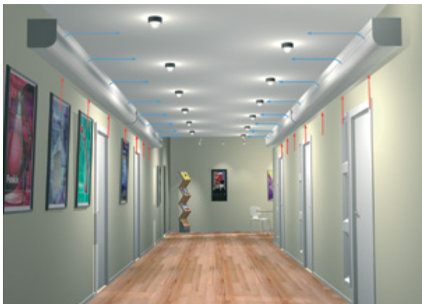
Picture 5. Plafond C with air injection across the ceiling.
