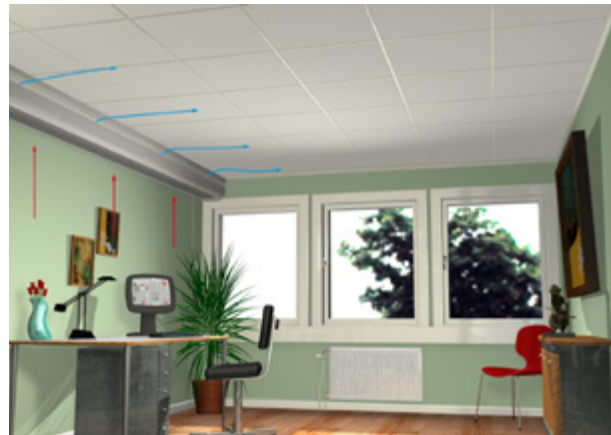
Picture 6. Plafond C with air injection across the ceiling.
