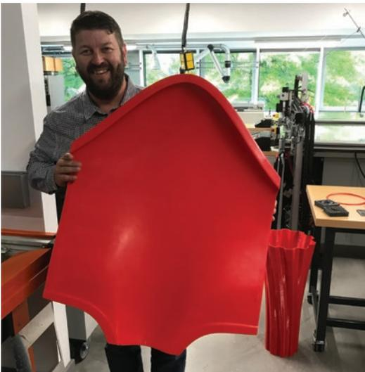
Utilizing a WorkSeries large format 3D printer from 3D Platform, the students were able to print the mold masters required for the drone in one piece. This eliminated the need for heavy fasteners or connectors to hold pieces together, and helped the craft to remain light enough in order to generate speed. The larger format also allowed for a larger wing span to generate more lift.
