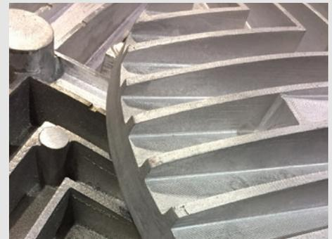
On the right is the 3D-printed PLA piece, with the first run aluminum casting on the left.
