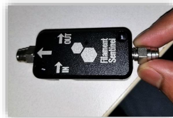
1. Remove the fitting at the entrance to the sensor (bottom of sensor).
