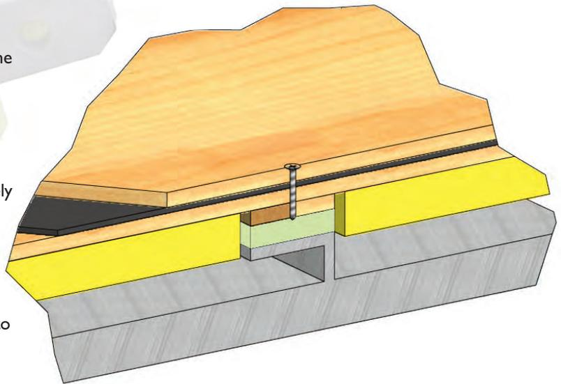
Typical installation of a floated sole on R-12 over a stiffened tank top.
