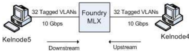
**Figure 2. Host-to-Host Test Setup**
