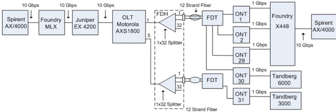
Figure 9. Test Setup: Different ONT, Different OLT Blade
