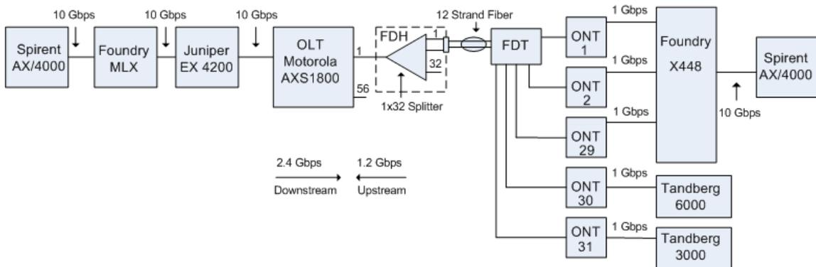
**Figure 8. Test Setup: Different ONT, Same OLT blade**
