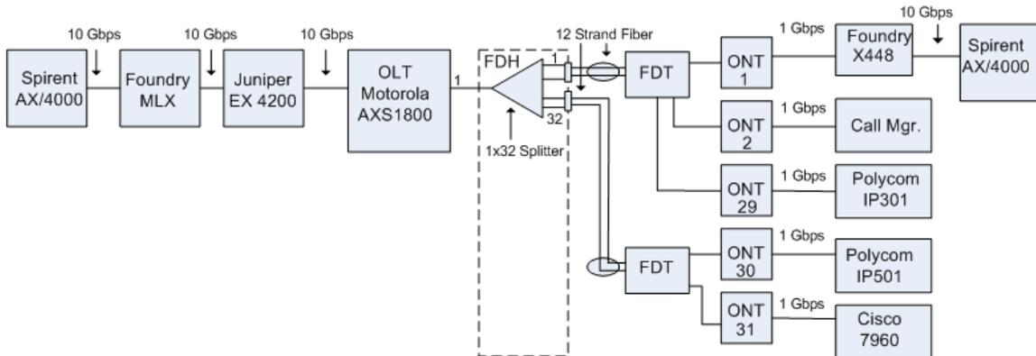
**Figure 10. VOIP Test Setup**
