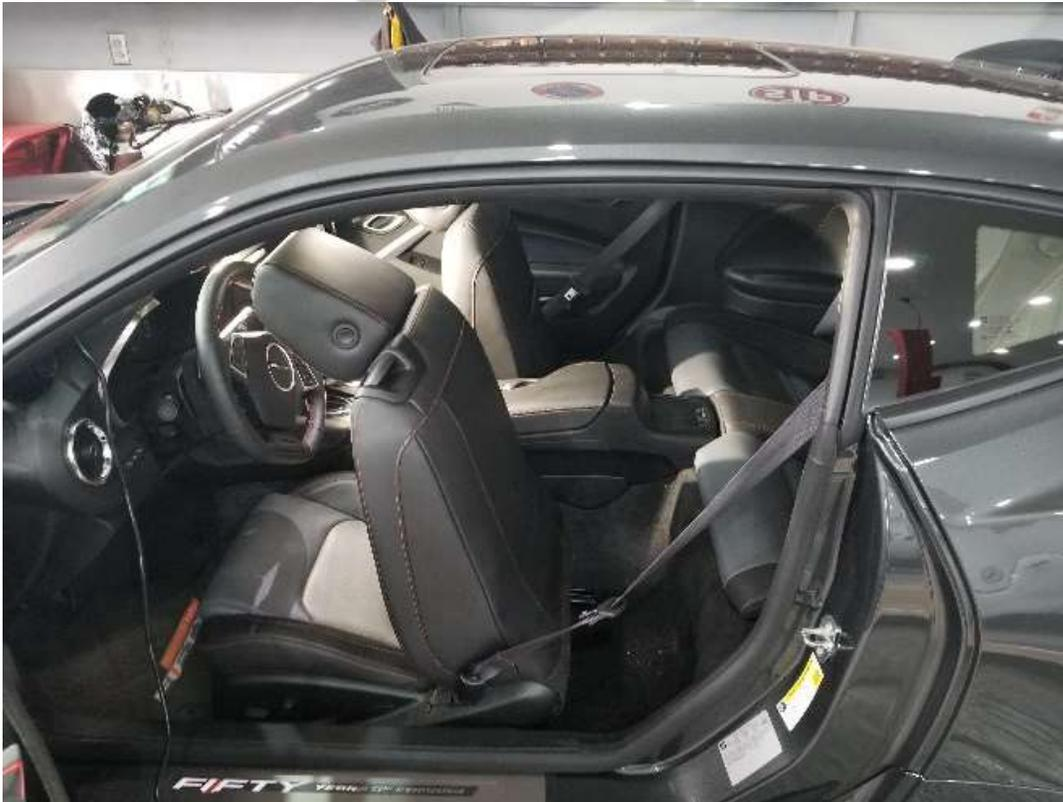
2. Starting on either side of the car, fold down the rear seatback and grasp with your hand, the lower seatback near the edge and lift. The seatback should raise out of the slot where it hinges. Its ok to use a bit of force is necessary to make it pop loose.
