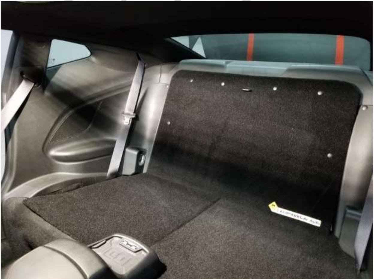
9. For a finished look we've included 3 matching carpet swatches to fill in the gaps left from removing the seats. One covers the passenger side panel groove where you can see your main power cable, the other two smaller sections can be inserted to cover the hinge opening from the seatback.
