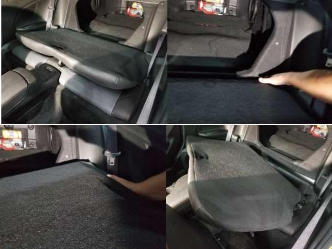
3. Move to the opposite side of the car and do the same lifting motion to remove the remaining side, lift the now free seatback out of the car and set aside.
