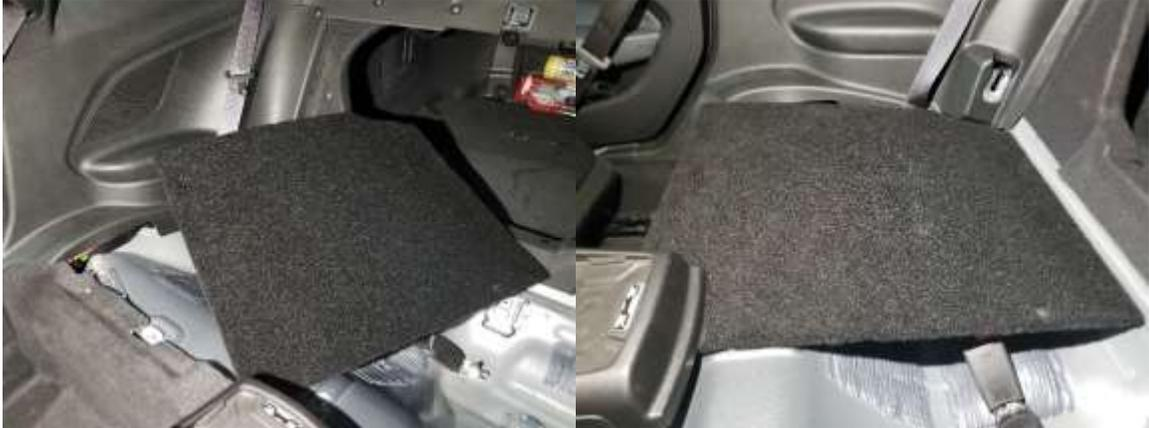
8. Align both panels so that the center seam is minimized and they both sit flush on the small lip just below the rear seatback panel. The contours of the side panels and the pressure placed on the front from the console will hold the lowers securely in place. Once done it will look like this:
