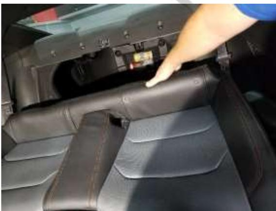
You can also grasp the front center of each seat bottom and feel where the retaining clip is located and pull up there to release it. This method does take significant force but again it will pop loose.
