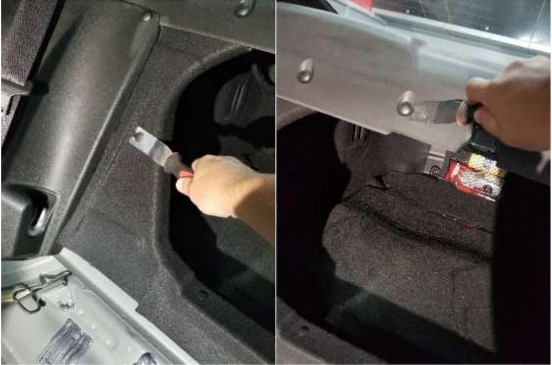
2. Once you have all 6 clips out, take your upper seatback and orient it so that the correct side faces forward (Unfortunately it's impossible to not have seams on a fully carpeted panel, however we've made sure the unsightly seams are all on the back to leave the most attractive side facing the passenger compartment). Place the panel into position using the upper protruding seatback loop as your guide.
