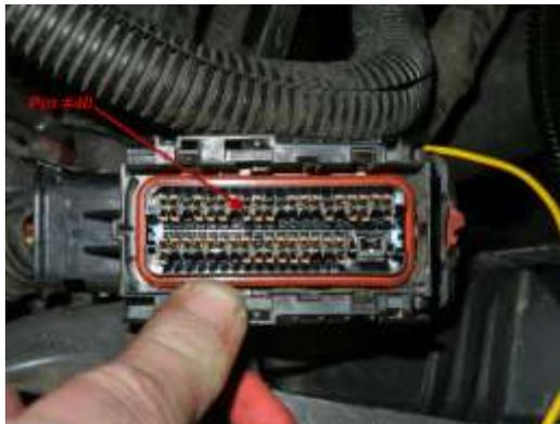
Another view of the terminal once made flush, note the orientation of the terminal is the same as the others
