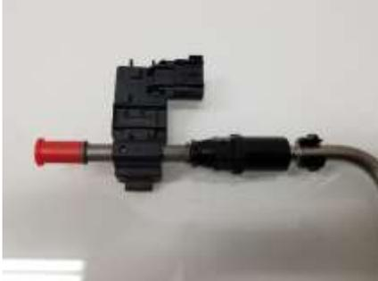
5. Next remove red shipping cap (if equipped) from sensor module tube and then connect the flexible tube onto the sensor, you should feel it click into place. And it will look similar to the image below.
