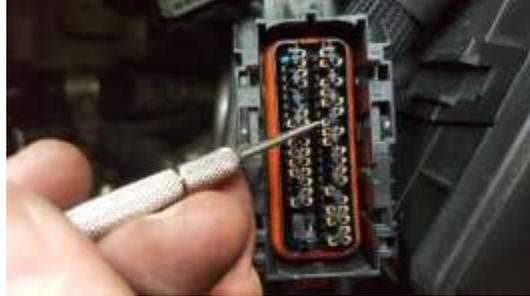
Same plug with the plastic terminal cover removed to expose the terminals and ensure the signal wire gets seated
