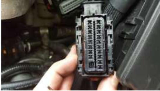
Cover installed (shown above) here protects the terminals
