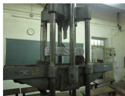
Figure 3: Testing of Pervious Concrete
