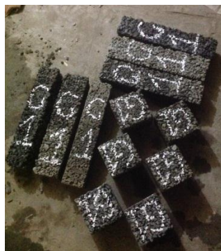
Figure 2: Specimens of Pervious Concrete
