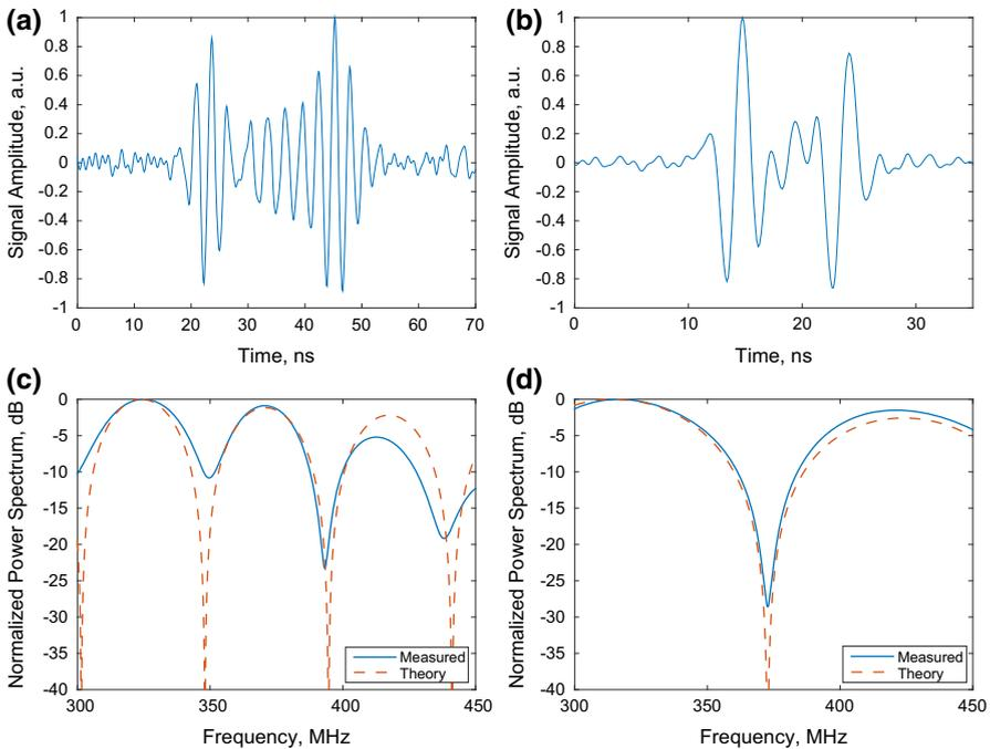
**Fig. 2** Measured A-lines from an US pulse backscattered by a cell (a) and PA signal emitted by the nucleus of the same cell (b). The power spectra of the backscattered US pulse and the best-fit spectrum generated using Eq. 2 and photoacoustic signal and the fit power spectrum of Eq. 9 are shown in (c, d), respectively. The power spectra were windowed to match the transducer bandwidth
