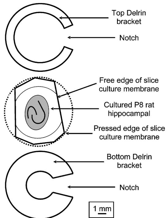
Fig. 1. Schematic of assembly used to obtain MRI of rat hippocampal slice cultures. The slice culture and attached membrane are cut away from the cell culture inserts and trimmed to fit inside a 10-mm NMR tube (inner diameter  $\sim 9$  mm). The edges of the culture membrane then are pressed between the top and bottom Delrin brackets. Notches in the Delrin brackets are used for passage of a Delrin anchor, which can then be used to remove the sample after imaging is complete.
