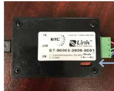
Ensure the RX switch found on the back of your Link Kit is set to position 2 for Cyclops.
