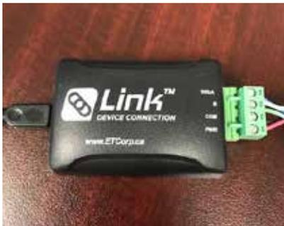
Double check to ensure physical wiring from the Cyclops sensor to the Link Kit is correct, and making proper contact.
