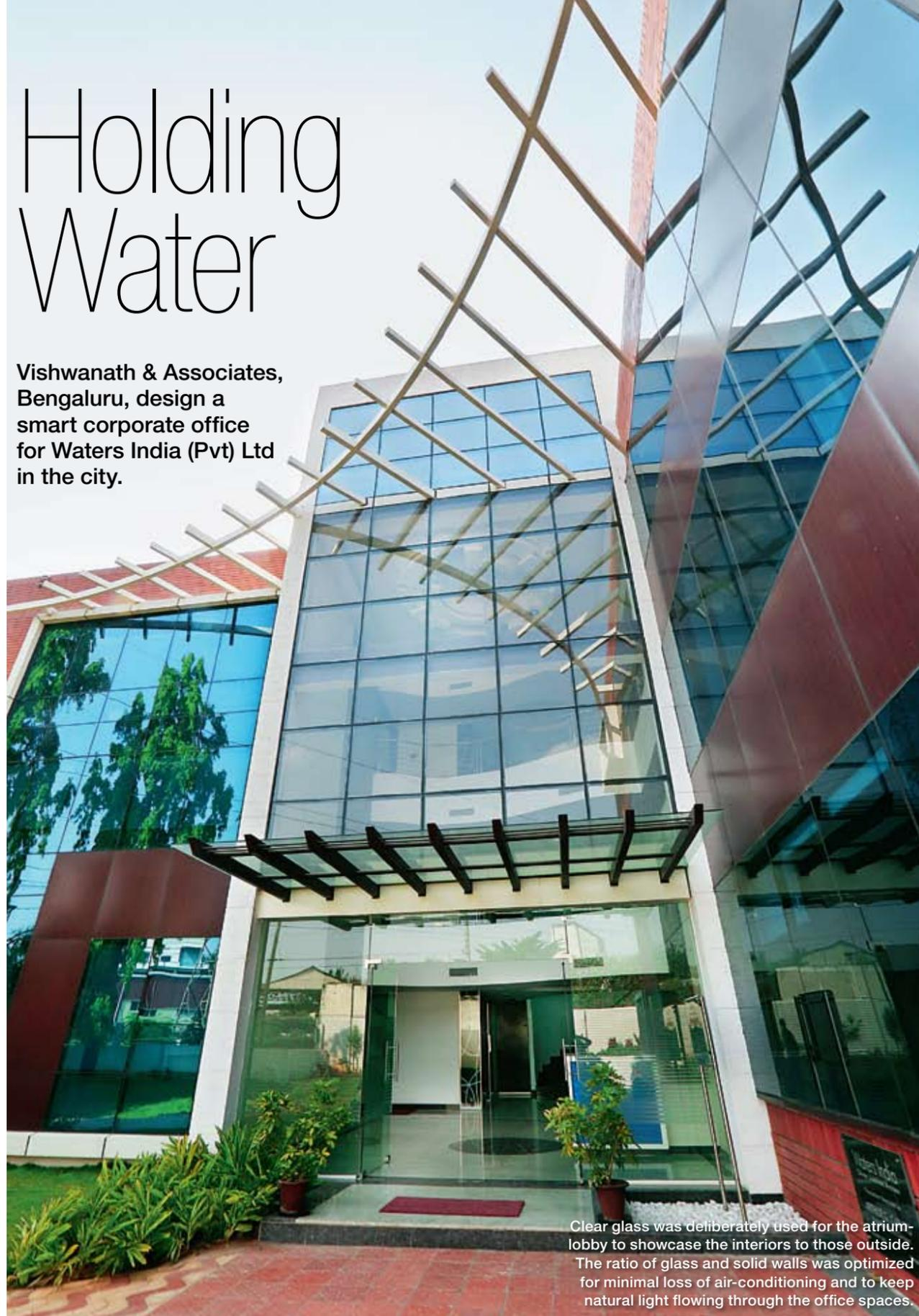
Clear glass was deliberately used for the atrium-lobby to showcase the interiors to those outside. The ratio of glass and solid walls was optimized for minimal loss of air-conditioning and to keep natural light flowing through the office spaces.
