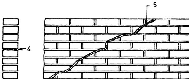
1B Cement mortar and flat chips in wide cracks
