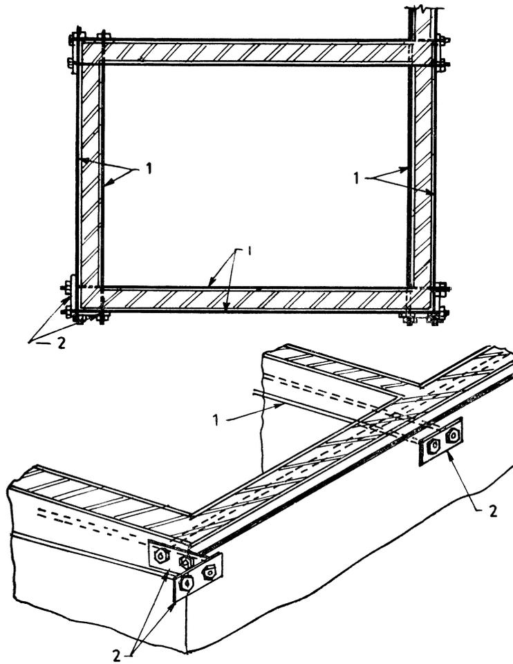
1. Steel rods for prestressing                      2. Anchor plates
