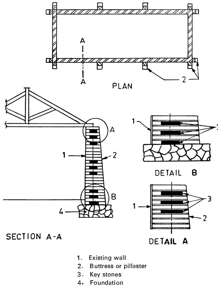
FIG. 14 STRENGTHENING OF LONG WALLS BY BUTTRESSES
