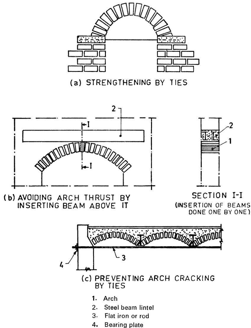
FIG. 13 STRENGTHENING AN ARCHED OPENING IN MASONRY WALL
