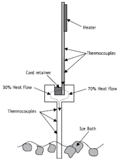
FIGURE 3 - THERMAL TEST APPARATUS SCHEMATIC DIAGRAM [6]
