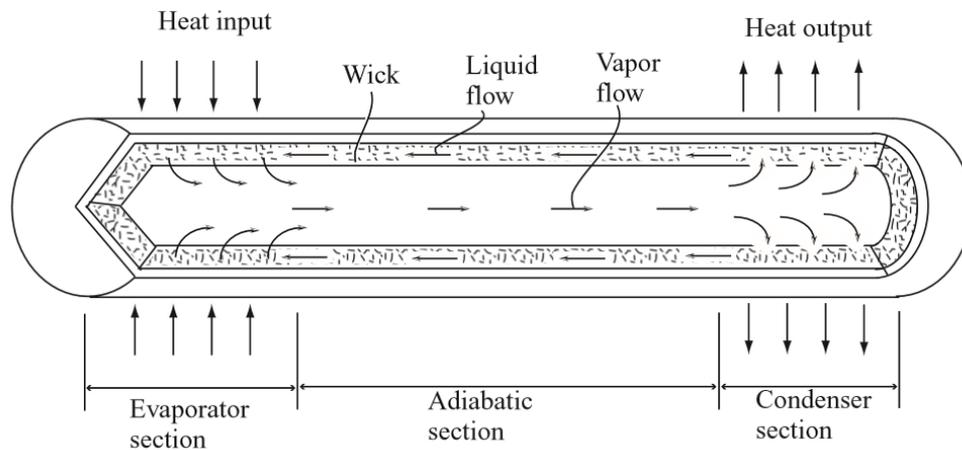
FIGURE 1 - CROSS SECTION OF A HEAT PIPE [2]
