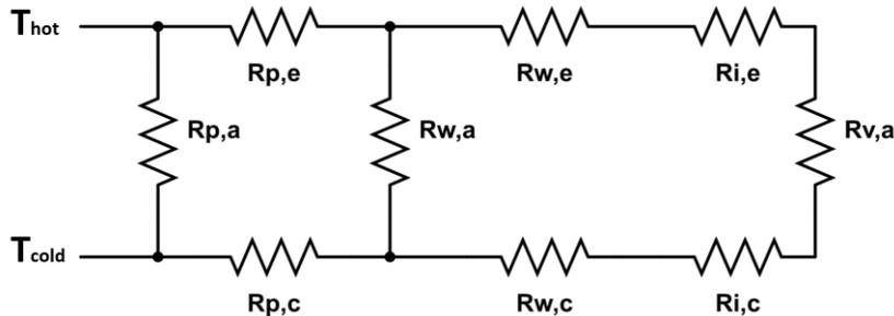
FIGURE 3 – ELECTROTHERMAL NETWORK OF A HEAT PIPE
