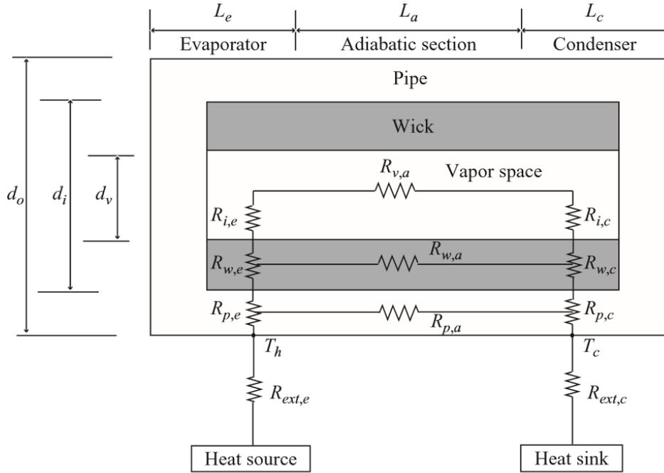
FIGURE 2 – HEAT PIPE THERMAL RESISTANCE NETWORK [2]
