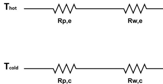
**FIGURE 4 – SIMPLIFIED ELECTROTHERMAL NETWORK OF A HEAT PIPE**
