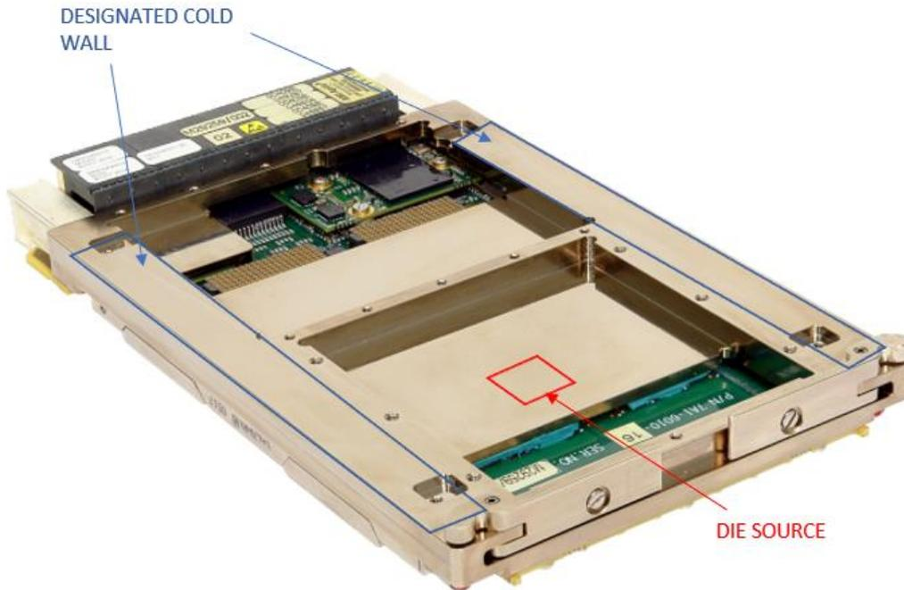
FIGURE 4 - VPX APPLICATION WITH HEAT SOURCE AND SINKS [3]
