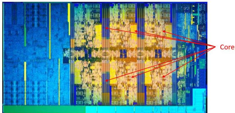
FIGURE 1 - DIE MAPPING OF INTEL 6 CORE ARCHITECTURE [1]
