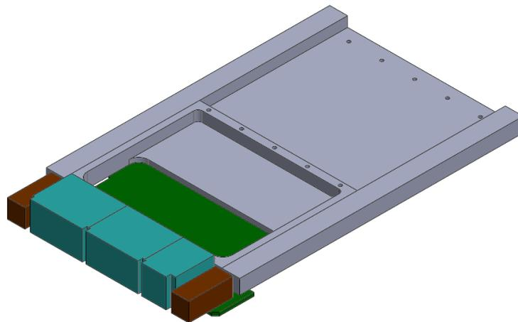
FIGURE 7 - MODEL OF A 3U CARD WITH SECONDARY THERMAL INTERFACE BARS REMOVED
