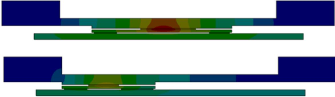
FIGURE 11 - A THERMAL PLOT THROUGH THE DIE JUNCTION IDENTIFYING THE DISTINCTLY DIFFERENT DISPERSION OF FLUX IN AN XMC CAPABLE HEATSINK
