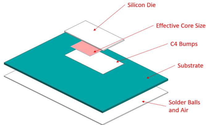
FIGURE 2 - EXPLODED VIEW OF A TYPICAL CPU CONSTRUCTION
