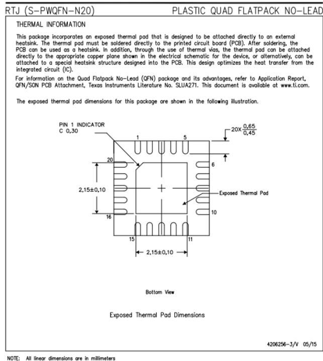
FIGURE 4 - DEVICE DRAWING OF TI SATA REDRIVER [4]
