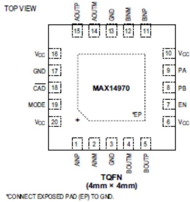
FIGURE 5 - DEVICE DRAWING OF MAXIM SATA REDRIVER [5]
