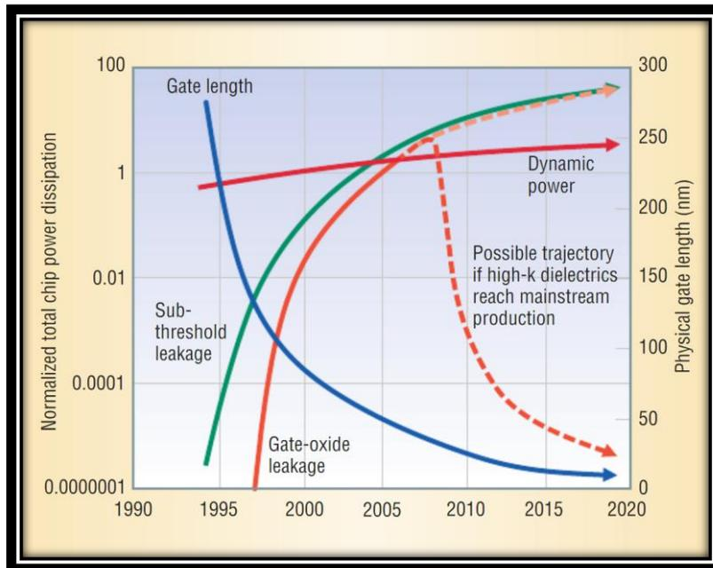
FIGURE 2 - TOTAL CHIP DYNAMIC AND STATIC POWER DISSIPATION TRENDS ITRS [7]
