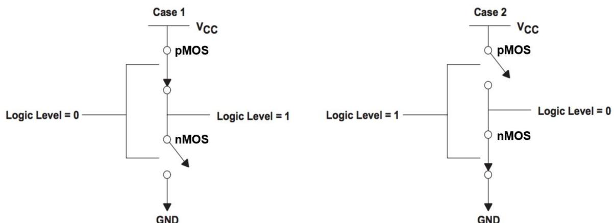
FIGURE 1 - CMOS INVERTER MODE FOR STATIC POWER CONSUMPTION [6]
