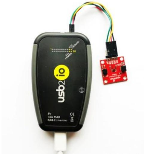
3. Turn VCCIO to necessary voltage, for example 3.3V: 'expv write 3300'.
