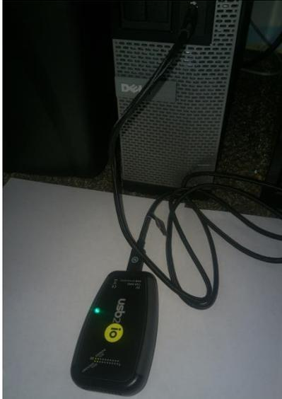
3. Check device manager (in Windows) for “USB Serial Device” or find ttyACMx device in Ubuntu Linux/MacOS.
