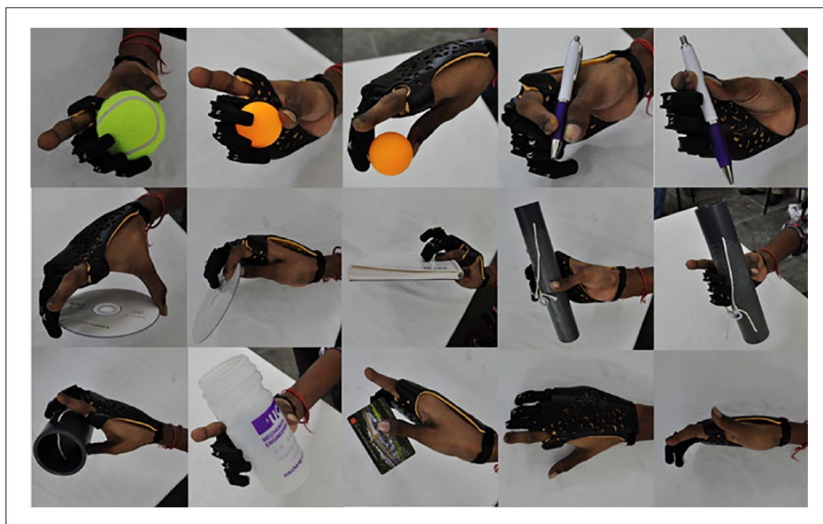
Figure 3. Demonstration of the grasp taxonomy test. 13 The grasps were divided into power and precision grasps. The use of index and thumb were minimized to ensure testing of the prosthesis itself.
