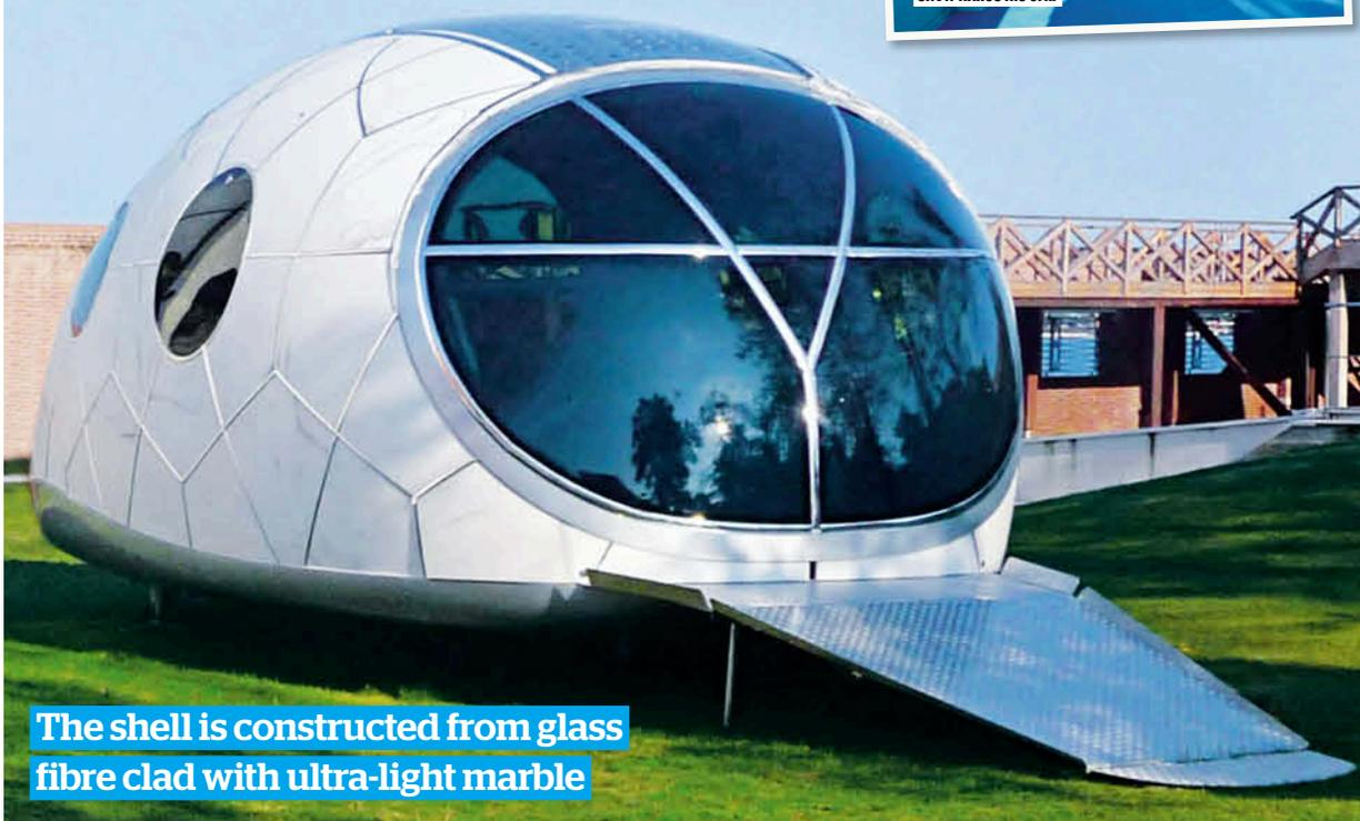
The shell is constructed from glass fibre clad with ultra-light marble
