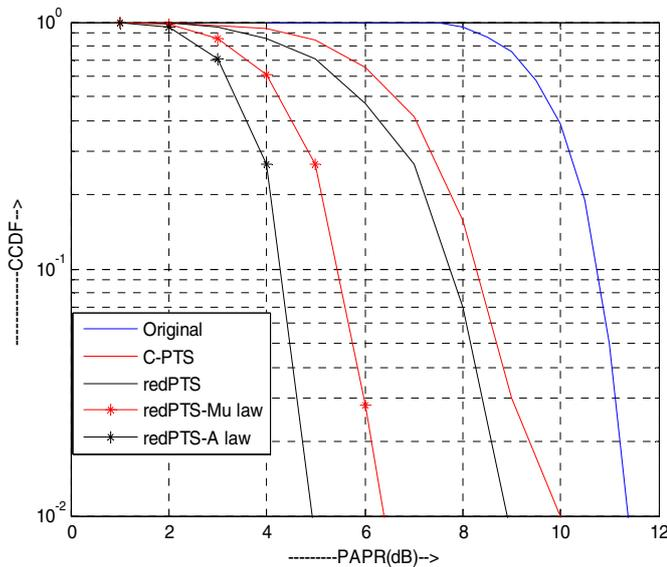
Fig. 4 comparison of PAPR for Reduced complexity PTS with companding OFDM system
