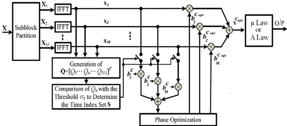
Fig. 3 Reduced complexity PTS with companding OFDM system
