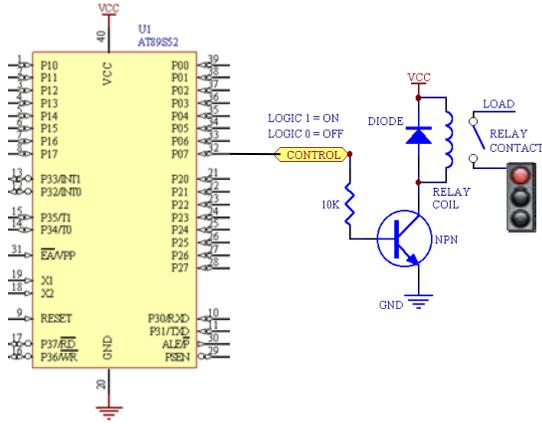
Figure. 4 Traffic Light Driving Relay Interface with Microcontroller.
