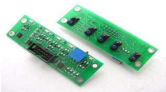
Figure. 2 TCRT Sensor Module [6]
