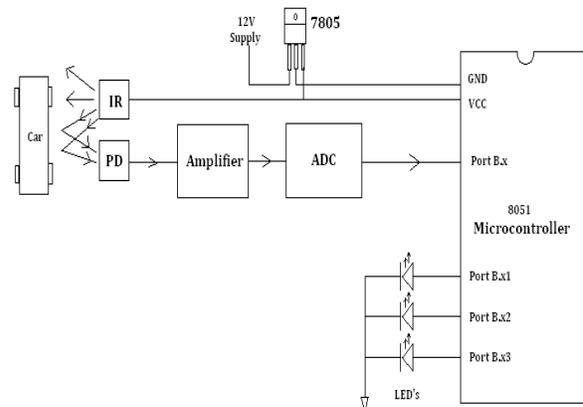
Figure. 3 Sensor Interface with Microcontroller.
