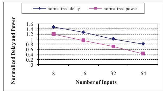
Fig. 7. Relationship between normalized delay and power consumption of proposed circuit in terms of number of inputs under same UNG.
