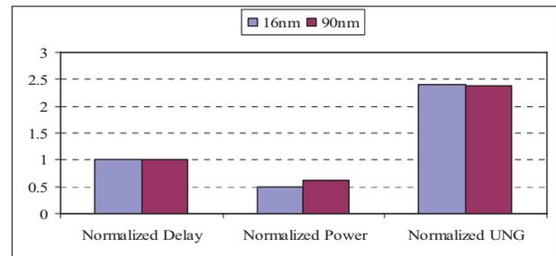
Fig. 8. Relationship between normalized delay, power consumption, and UNG of proposed circuit in two technology nodes.
