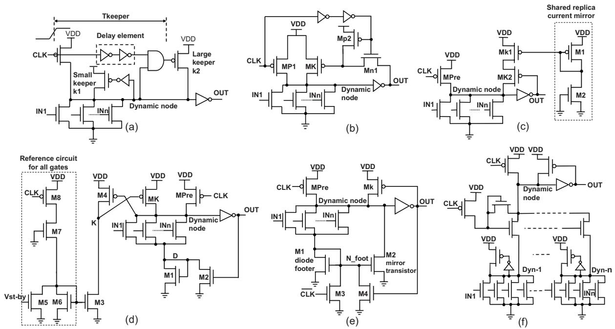
Fig. 2. (a) CKD [5]. (b) HSD [6]. (c) LCR keeper [7]. (d) CKCCD [8]. (e) DFD [4]. (f) DPD [9].
