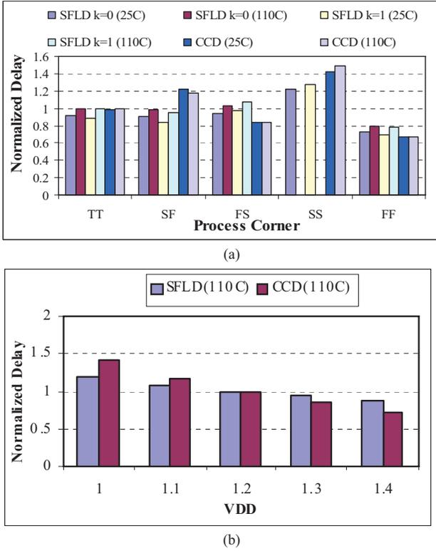
Fig. 9. Variation effects on the normalized delay of proposed circuit (CCD). (a) Process and temperature variation effects. (b)  $V_{DD}$  variation effect.
