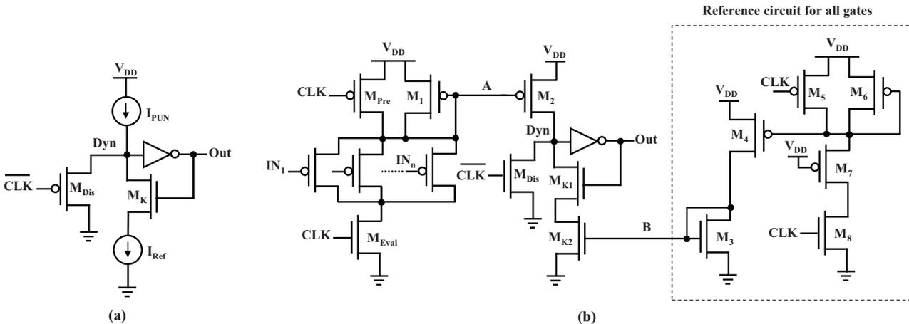
Fig. 3. (a) Concept of proposed circuit (CCD). (b) Implementation of wide OR gate using CCD.
