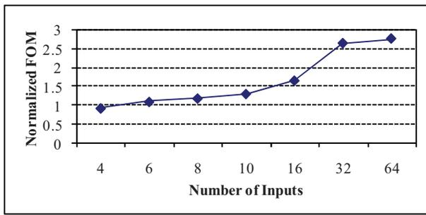
Fig. 6. Relationship between normalized FOM of proposed circuit and number of inputs.
