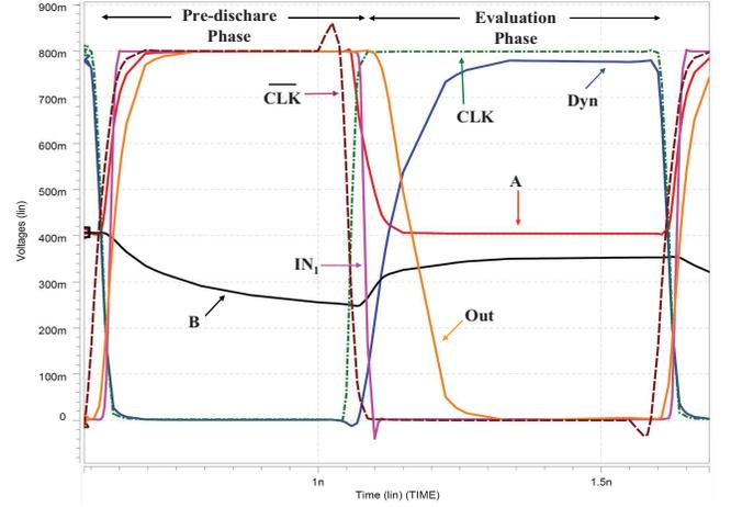
Fig. 4. Simulated waveforms of the 32-input OR gate implemented in the proposed domino circuit.
