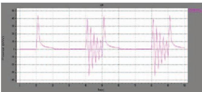
Fig.14. FinFET\_32 dynamic (switching) power of NOR gate.
