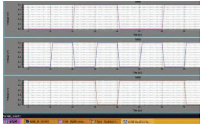
Fig.8. NAND gate Simulation result
