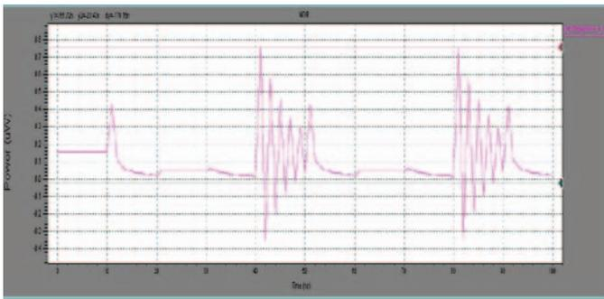
Fig.13. CMOS\_32 dynamic (switching) power of NOR gate.
