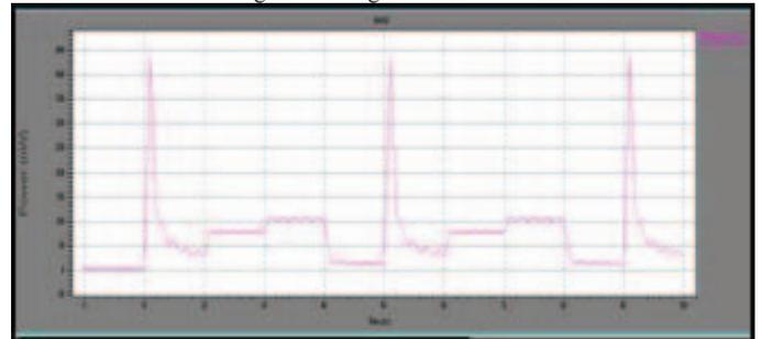
Fig.9. CMOS\_32 dynamic(switcing) power of NAND gate.
