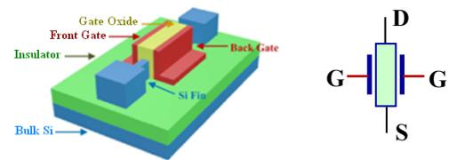
Figure 1. (a) Top view of double gate FinFET structure and (b) its symbol.
