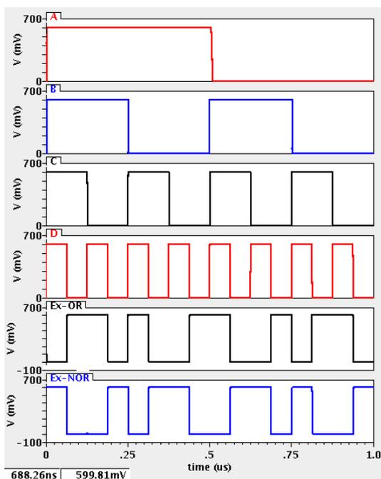
Figure 4. Input and output waveforms of 4-input XOR/XNOR Circuit
