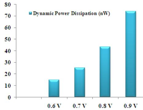
Figure 6. Simulated dynamic power dissipation Vs Voltage.
