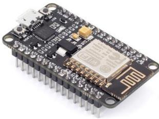
Figure 4: NodeMcu Microcontroller
