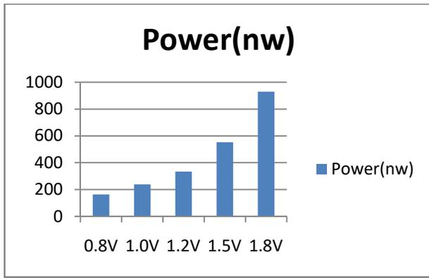
Fig. 8 Dynamic power variation of proposed full adder while varying the supply from 0.8V to 1.8V.
