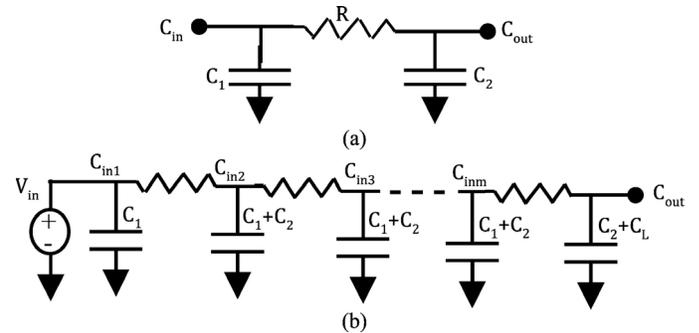
Fig.7 (a) R-C Equivalent of Transmission gate which causes delay, (b) R-C Equivalent of  $m$ -stage cascaded.
