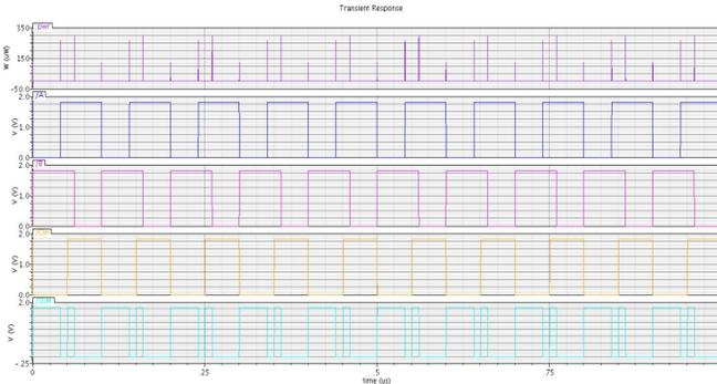
Fig. 5 Input Output wav form of proposed full adder at 1.8V supply
