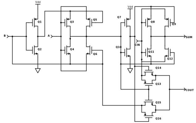
Figure. 2 Complete diagram of proposed full adder
