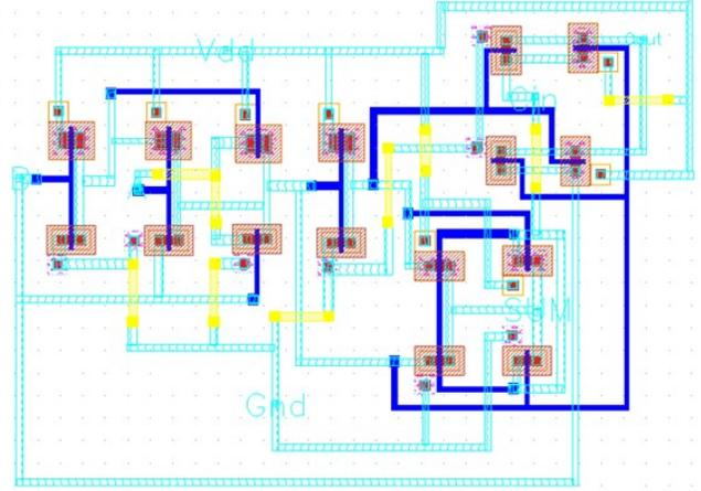
Fig. 6 Layout of Proposed Full Adder
