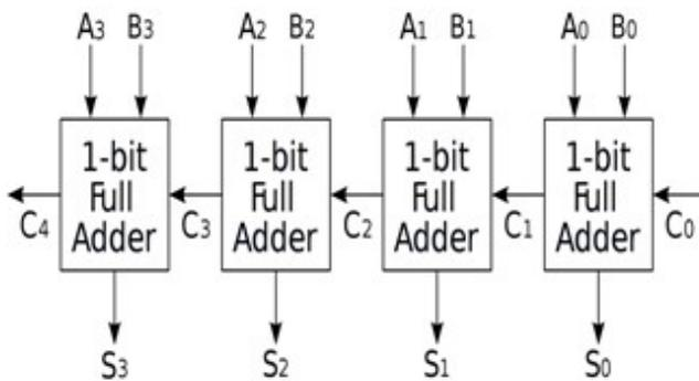
Fig. 9 Building block diagram of 4-Bit Ripple Carry Adder
