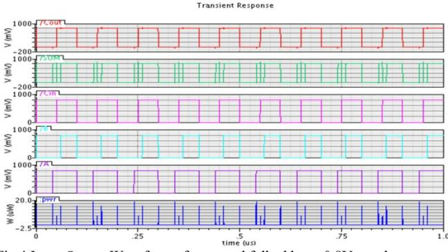
Fig.4 Input Output Waveform of proposed full adder at 0.8V supply
