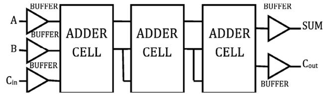
Fig.3 Three Stage Simulation test bench setup
